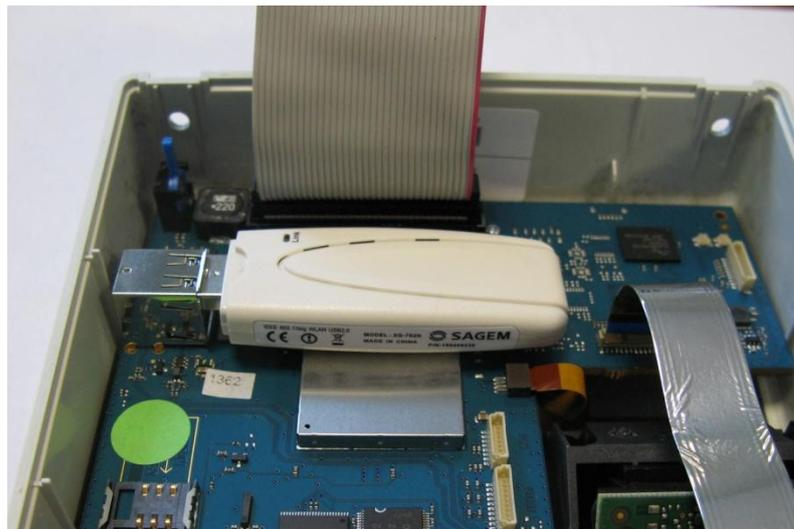
Figure 9: Installation adaptateur Wi-Fi™
